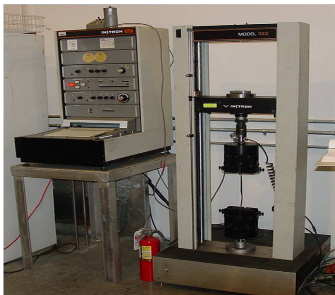
[Table/Fig-3]: Instron machine model no 1122 (Instron India Ltd)
